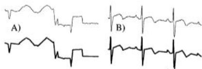
Fig. 1 Two time series and their piecewise linear representation. A) Space Shuttle Telemetry. B) Electrocardiogram (ECG)
